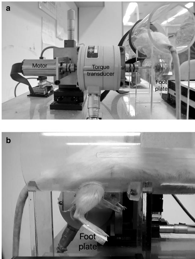
**Figure 2.** a. Instruments including brushless motor, torque transducer, and foot plate produced passive ankle motion and simultaneously measured resistant torque. b. Axis of the ankle joint was along with the rotational axis of the instruments.
