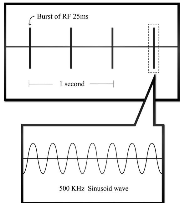
**Figure 4.** Electromagnetic waveforms of pulsed radiofrequency.
